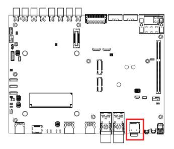
The external Micro SD card provides additional storage expansion. It is located behind the cover-plate on the front panel.
