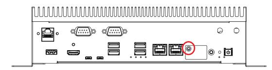
Step 2 Inserting SD card.
