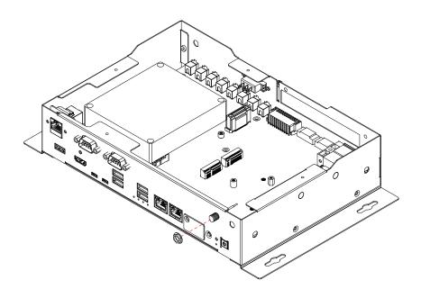
**Step 3** Fasten washer on the antenna cable connector.
