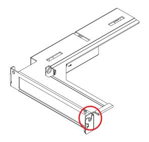
**Step 4** Install PCle card and fasten the screw indicated.
