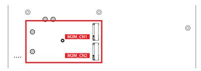
M.2 key M connector is suitable for applications that use Host I/Fs supported PCle x4, like w NVME Module card types include 2280.
