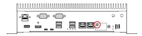
Step 2 Inserting SIM card, make sure the system power is not plugged.
