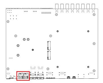
The external Nano SIM card offers wireless communication capability to the system.
