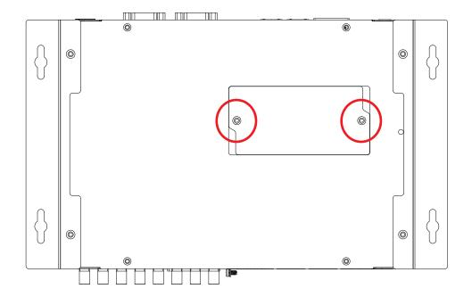
**Step 2** Install M.2 Key M 2280 into slot and fasten one pan head M3x4L screw.
