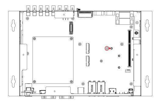
Step 2 Install M.2 Key B 3052 into slot and fasten one pan head M3x4L screw.
